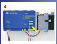
Wiring of the temperature sensor
