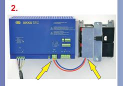
Connect the battery to the battery connector of the AKKUTEC
