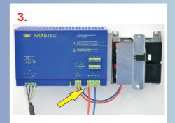
Connect the load to the buffered 24 V DC output to the AKKUTEC
