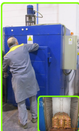
SHUNT 4000A - HEAT TREATMENT OVEN
