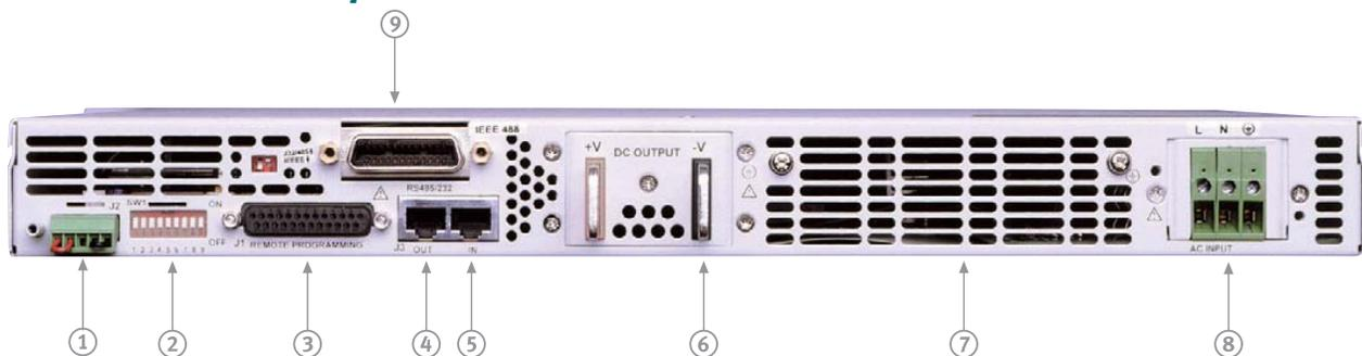
1. Remote/Local Output Voltage Sense Connections
