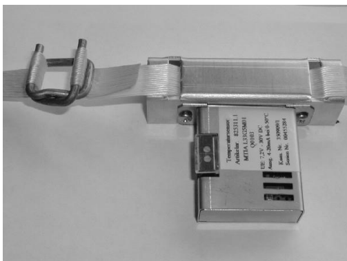
Fig. 2 installation at an external battery
