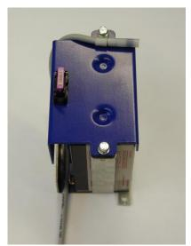
The battery sensor should be mounted near the battery, as in the example of the battery module NBBH 2402 (see picture). This ensures accurate measurement of the ambient temperature of the battery
